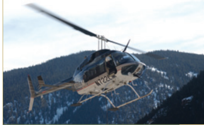
Above: The pilot carefully maneuvers a jet-powered Bell 206 L-4 Long Ranger over the chain link section where the ground crew attaches it for hoisting. The pilot is the only person on board to keep weight low at this high altitude. Inset: The chopper carefully lifts the heavy mesh before heading across I-70 to the rock fall mitigation area. High winds, common in mountainous areas, can challenge aerial deliveries even for experienced pilots. Below: The chopper pilot deftly lowers the mesh over the steel framework.
