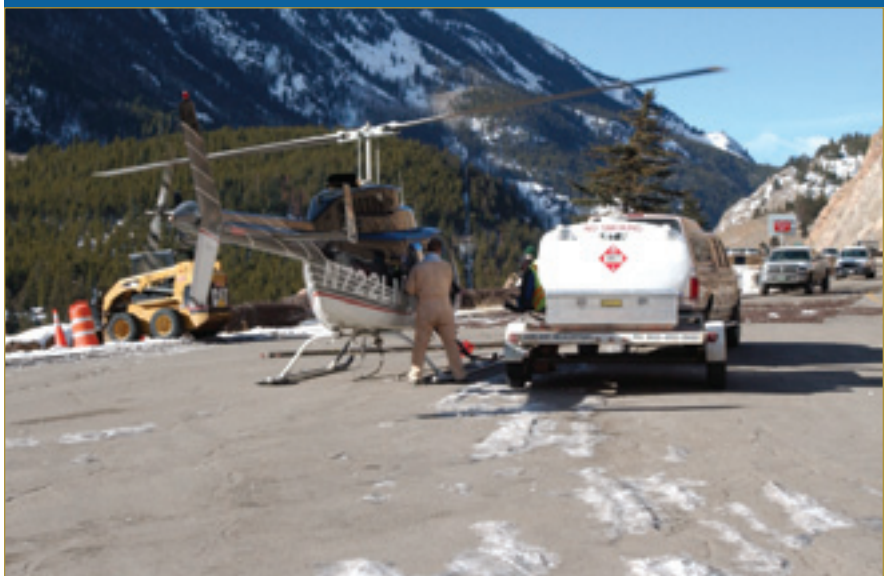
Above: Between airlifts of mesh, approximately 15 minutes apart, aviation crew refuels the helicopter with only 10 gallons of jet fuel to keep gross weight down.
